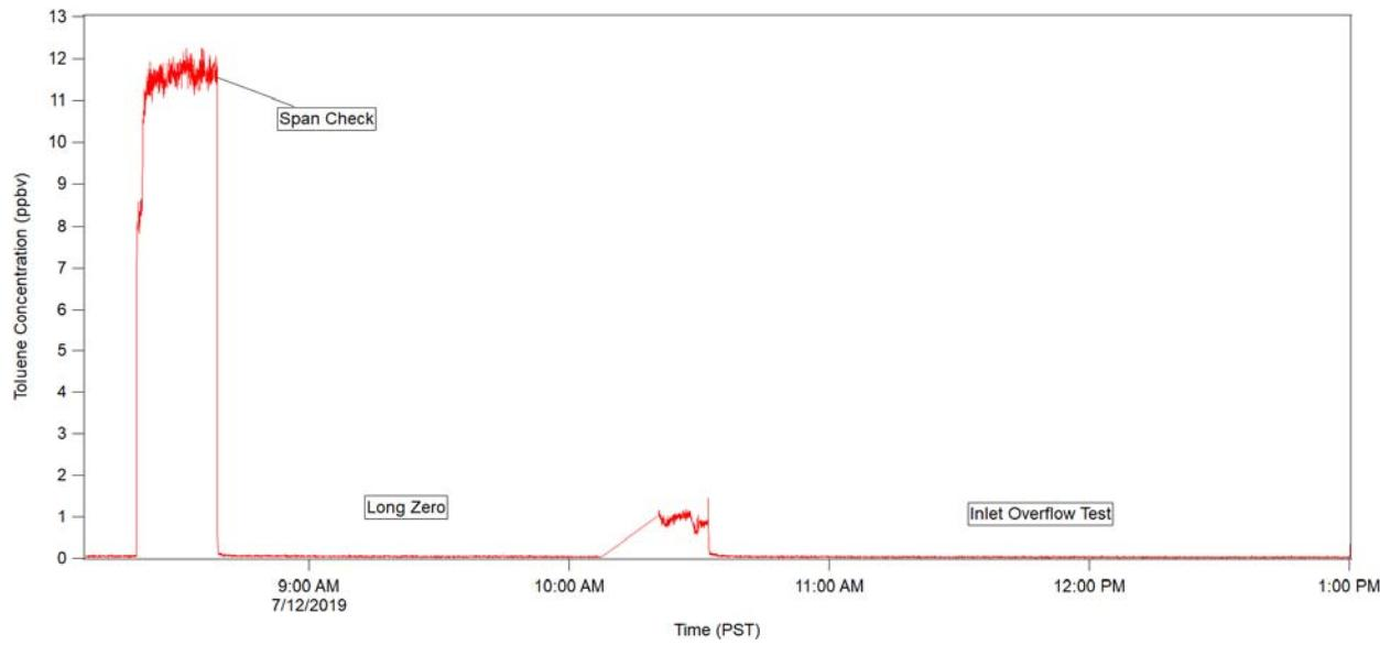
**Figure 6-1. Proton Transfer Reaction – Mass Spectrometer Testing; Span Check, Long Zero, and Inlet Overflow on Toluene.**
