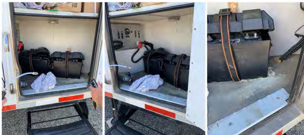
Figure 2-15. Sampling Setup for Monitoring the Emissions from the Trailer Emitting Strong Odors and Containing Overcharged Batteries Located on the East Side of AP Farm.
