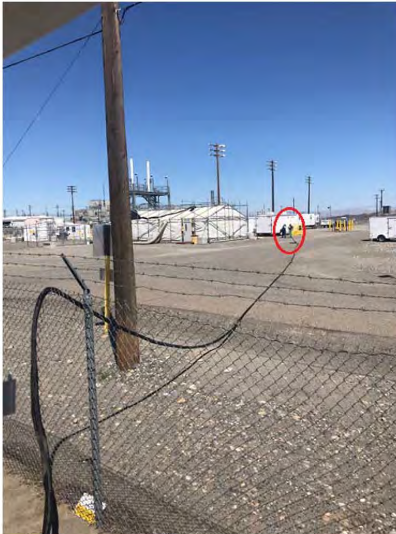
Figure 2-3. Mobile Laboratory 208-foot Heated Line Placement During June 19, 2019, AOP-015 Event (Inlet Stand Circled in Red).
