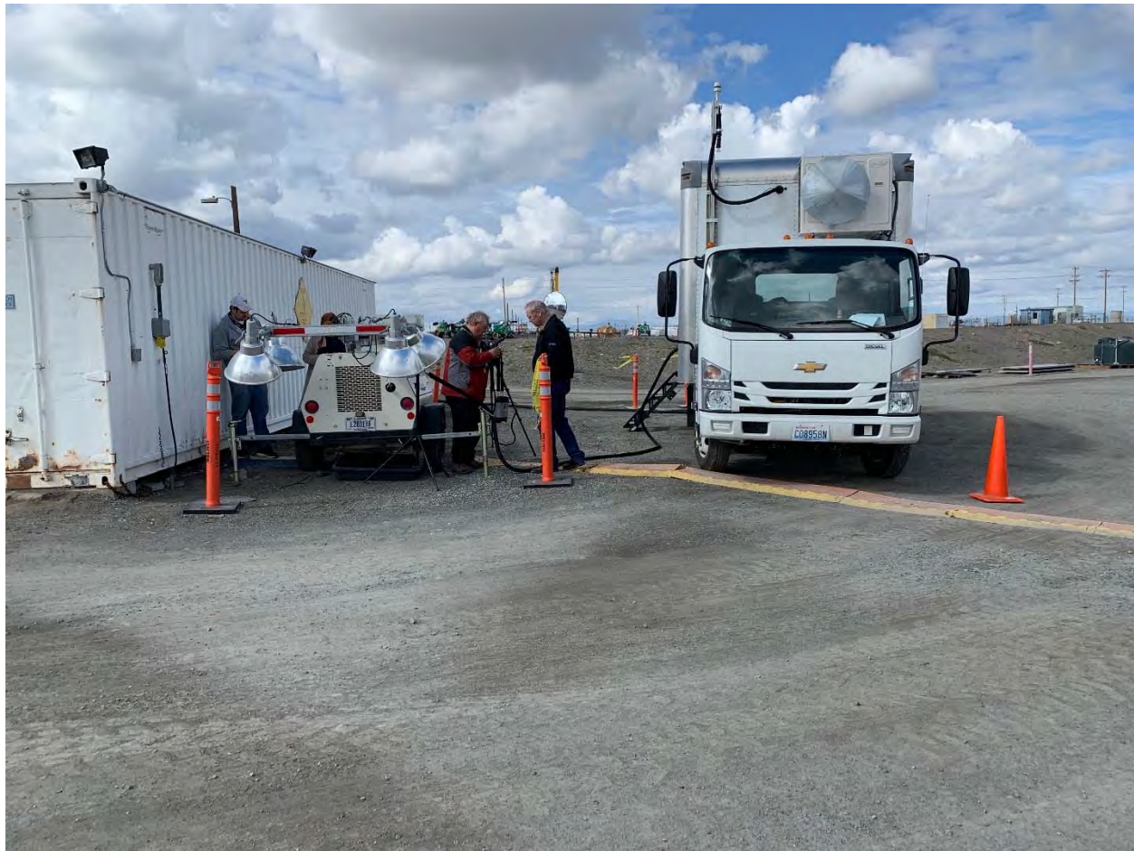
Figure 5-3. Mobile Laboratory Monitoring of Generator #2.
