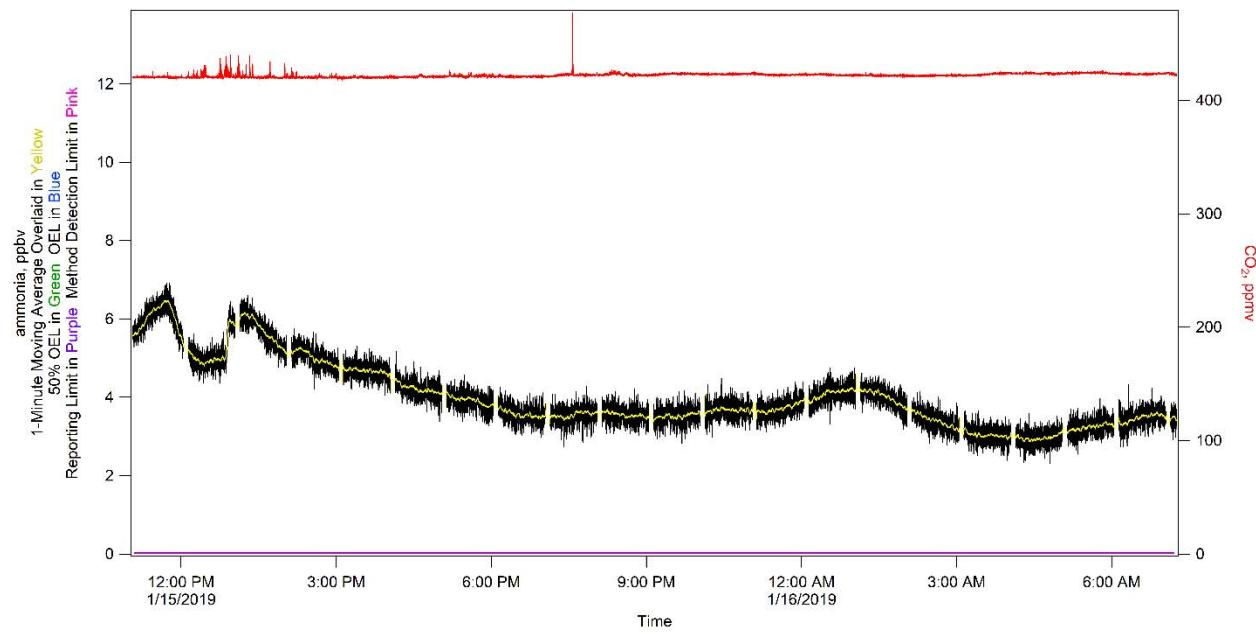
**Figure 3-3. Ammonia.**
