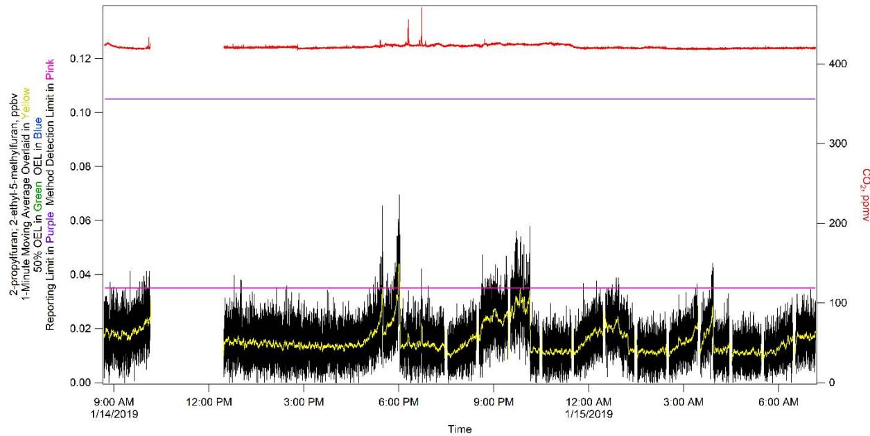
**Figure 2-11. 2-propylfuran + 2-ethyl-5-methylfuran.**
