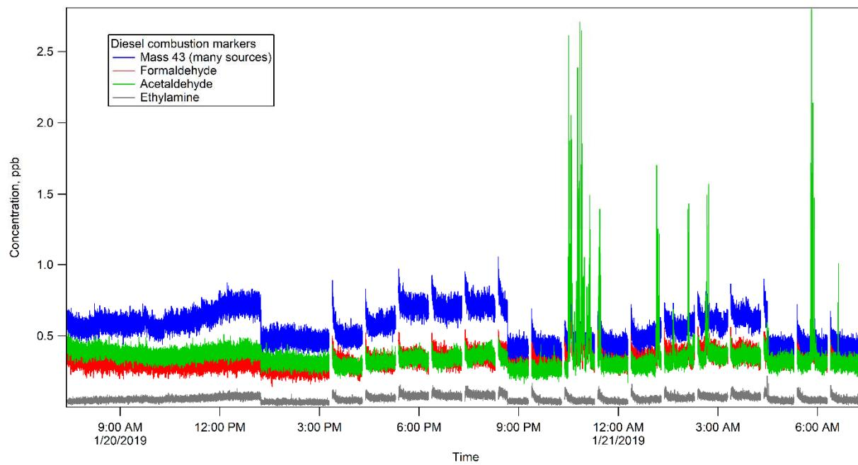
**Figure 8-19. Diesel Combustion Markers.**
