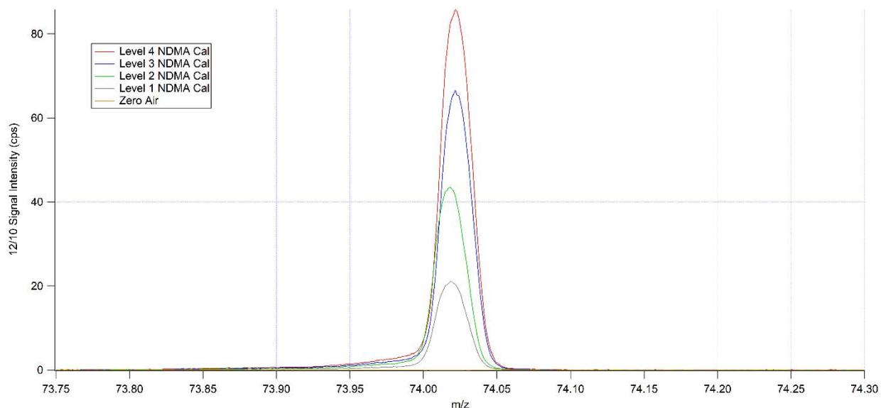
**Figure 1-4. Average Mass Spectra at m/z 74 for NDMA at Multiple Calibration Levels in NO<sup>+</sup> Mode.**
