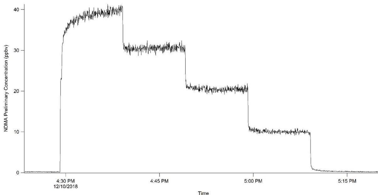
**Figure 1-5. Preliminary Time Series Plot of NDMA at Multiple Calibration Levels in NO<sup>+</sup> Mode.**
