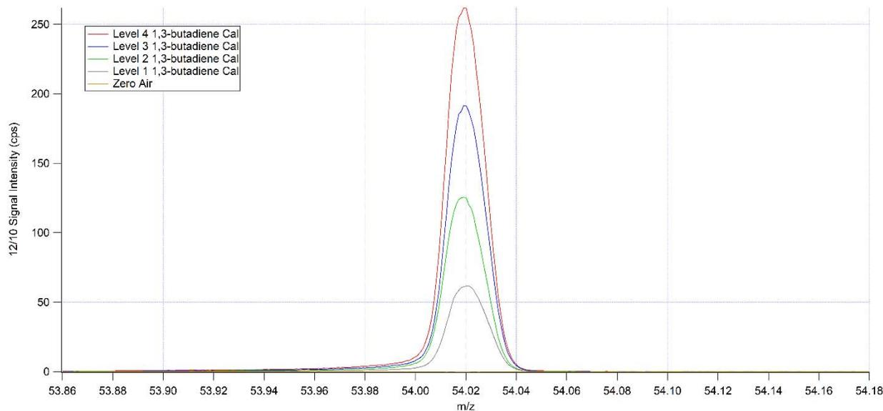
**Figure 1-2. Average Mass Spectra at  $m/z$  54 for 1,3-butadiene at Multiple Calibration Levels in  $\text{NO}^+$  Mode.**
