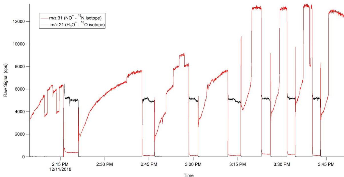
**Figure 2-1. Time Series Plot of Raw Counts of Reagent Ion Isotopes While Switching Between  $\text{NO}^+$  and  $\text{H}_3\text{O}^+$  Modes.**
