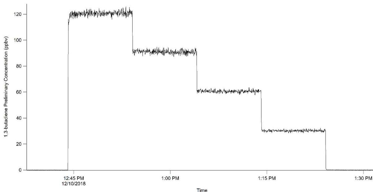
**Figure 1-3. Preliminary Time Series Plot of 1,3-butadiene at Multiple Calibration Levels in  $\text{NO}^+$  Mode.**
