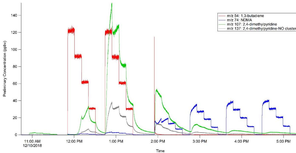
**Figure 1-1. Time Series Plot of Analytes of Interest for Calibration Sequences Performed on December 10, 2018.**
