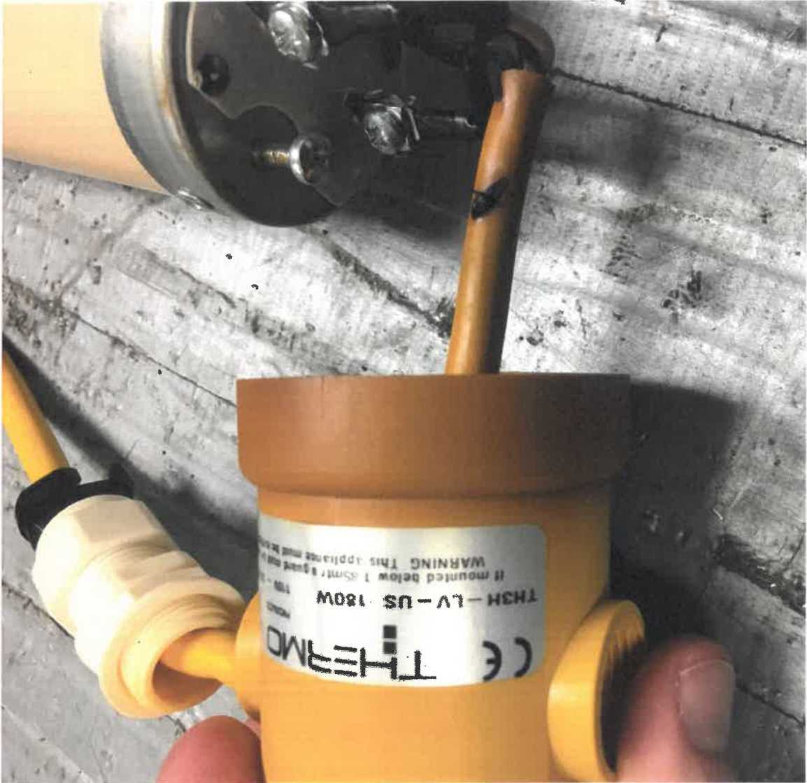
Figure 5: Discolored End Cap and Partially Melted Outer Cord Covering
