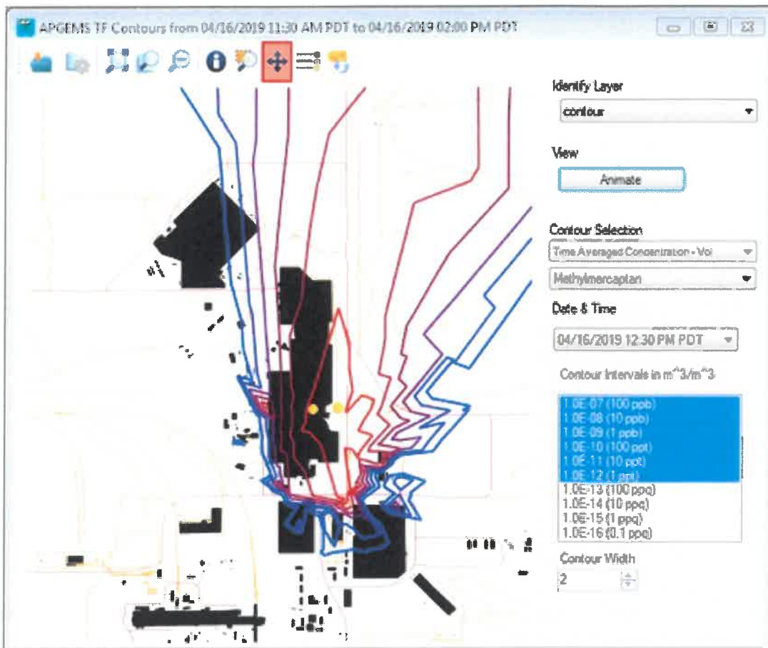
Figure 6. APGEMS-TF Model result from the two dumpster locations near the 242A Evaporator and 272AW near the time of the AOP-015 Event. Methyl mercaptan emission rate was 1 g/s from each of the two dumpsters.
