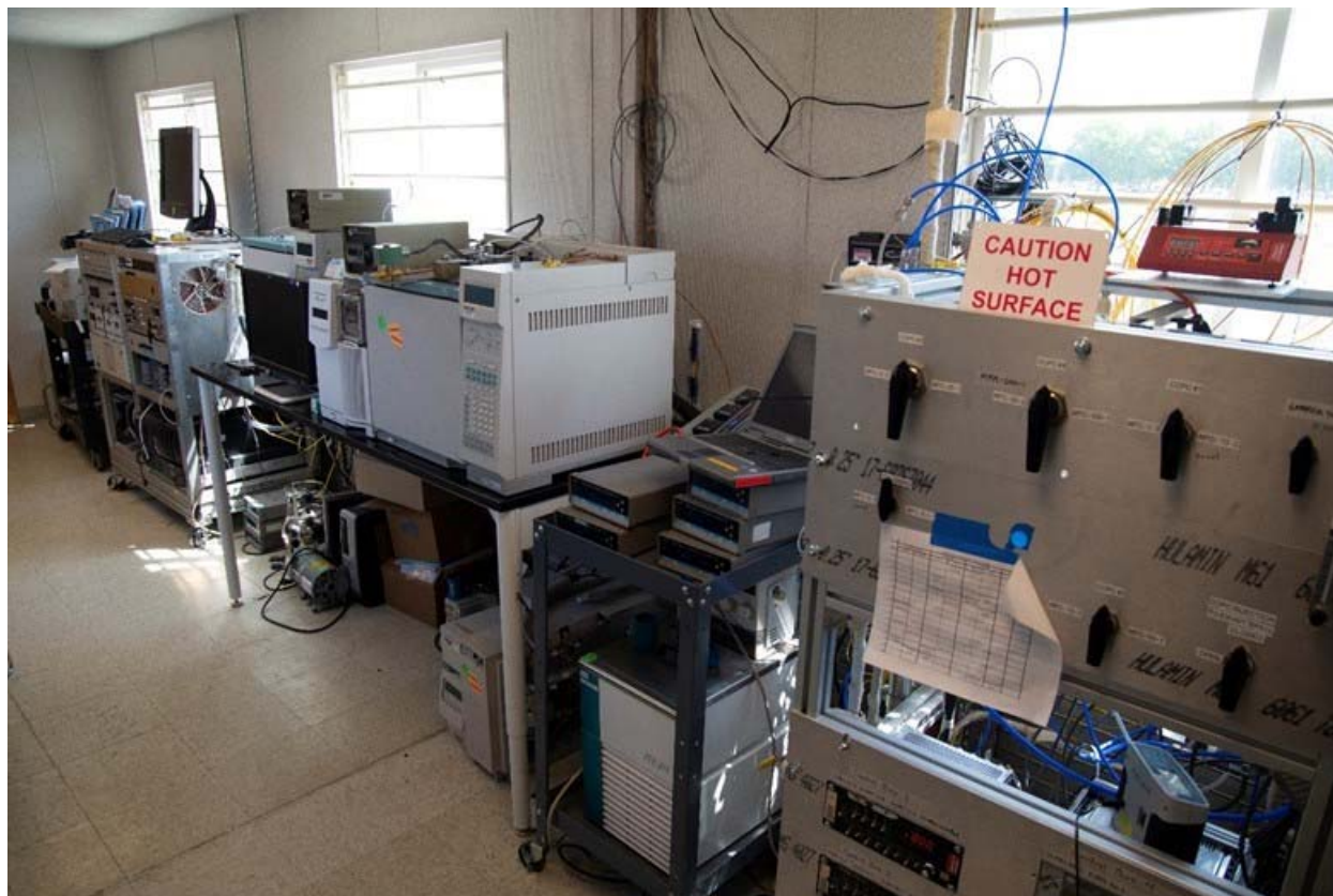
Figure B.1. Most of the instrumentation was along the east wall of the trailer. (Left to right) MKS FTIR, PTR-MS, the GC for pre-concentration (not used), the GC-MS (not used), the spare pumps and Mass Spectrometer (under the table and not used), heat tape controllers for the primary analytical sample loop lines (top of the cart), the chiller for sample temperature control (used only in the early testing), the injection system (top of the rack), and the sample collection controls (bottom of the rack).
