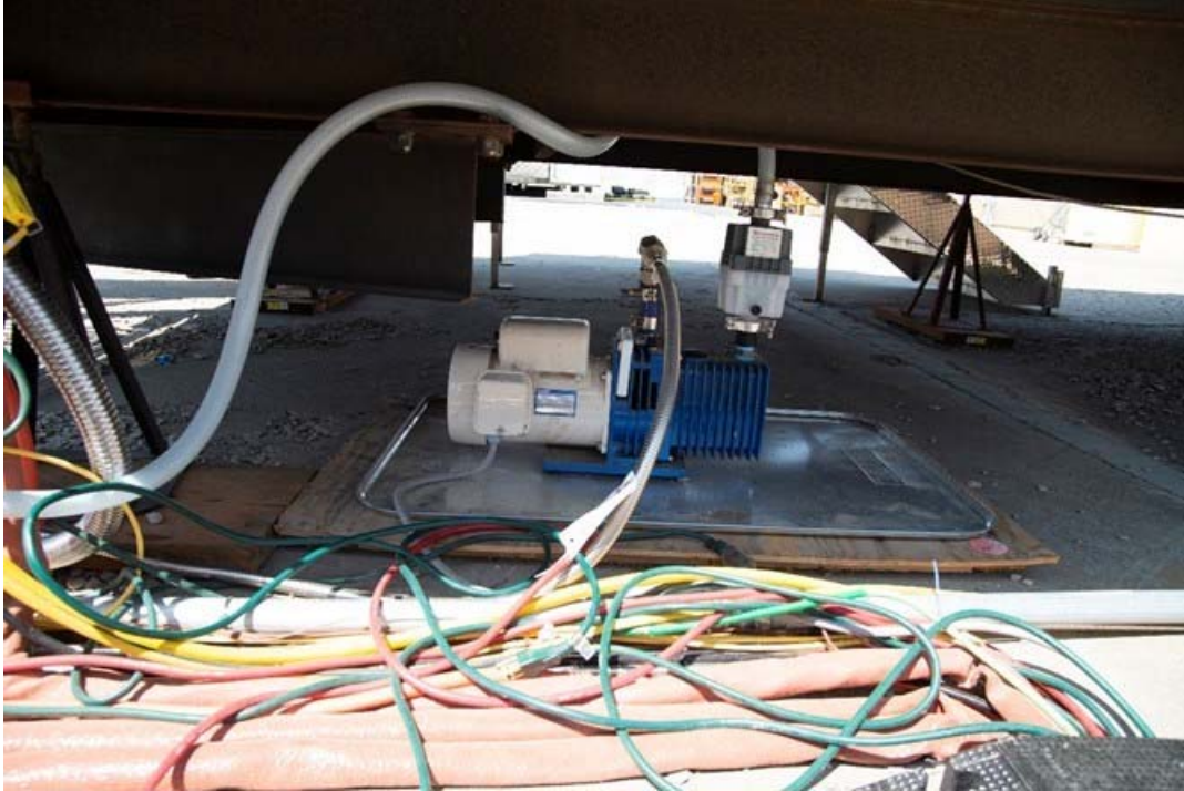
Figure B.8. In addition to the FTIR vacuum pump, a second vacuum pump was located under the trailer to supply mass flow controlled suction to the header, the media tubes, and for general cleaning gas sweeps.
