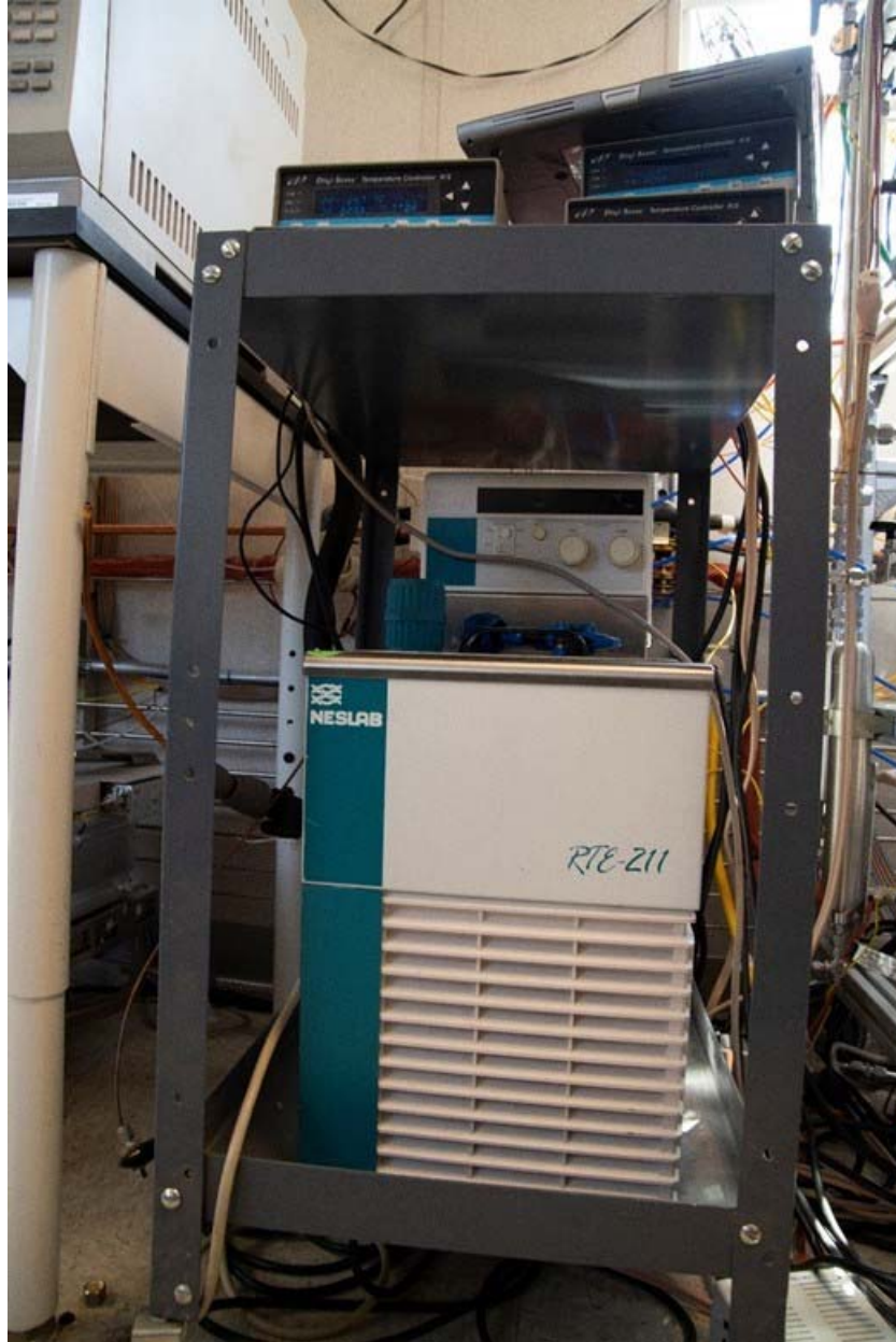
Figure B.5. The NESLAB RTE-211 was used to cool key sample lines as part of potential temperature controls along the exhaust sampling lines. It was used during shakedown and it was determined not to be necessary in later testing. The heat tape controllers on the top of the cart are part of the seven to ten tapes (depending on the test) that were operated at 120°C to 200°C during testing. They were on the primary analytical sample loop tubes and lines (as well as the intake sample lines) to limit moisture condensation as the exhaust cooled coming from the NUCON TOS. The orange insulation over the heat tape on the sampling header can be seen on the back wall.
