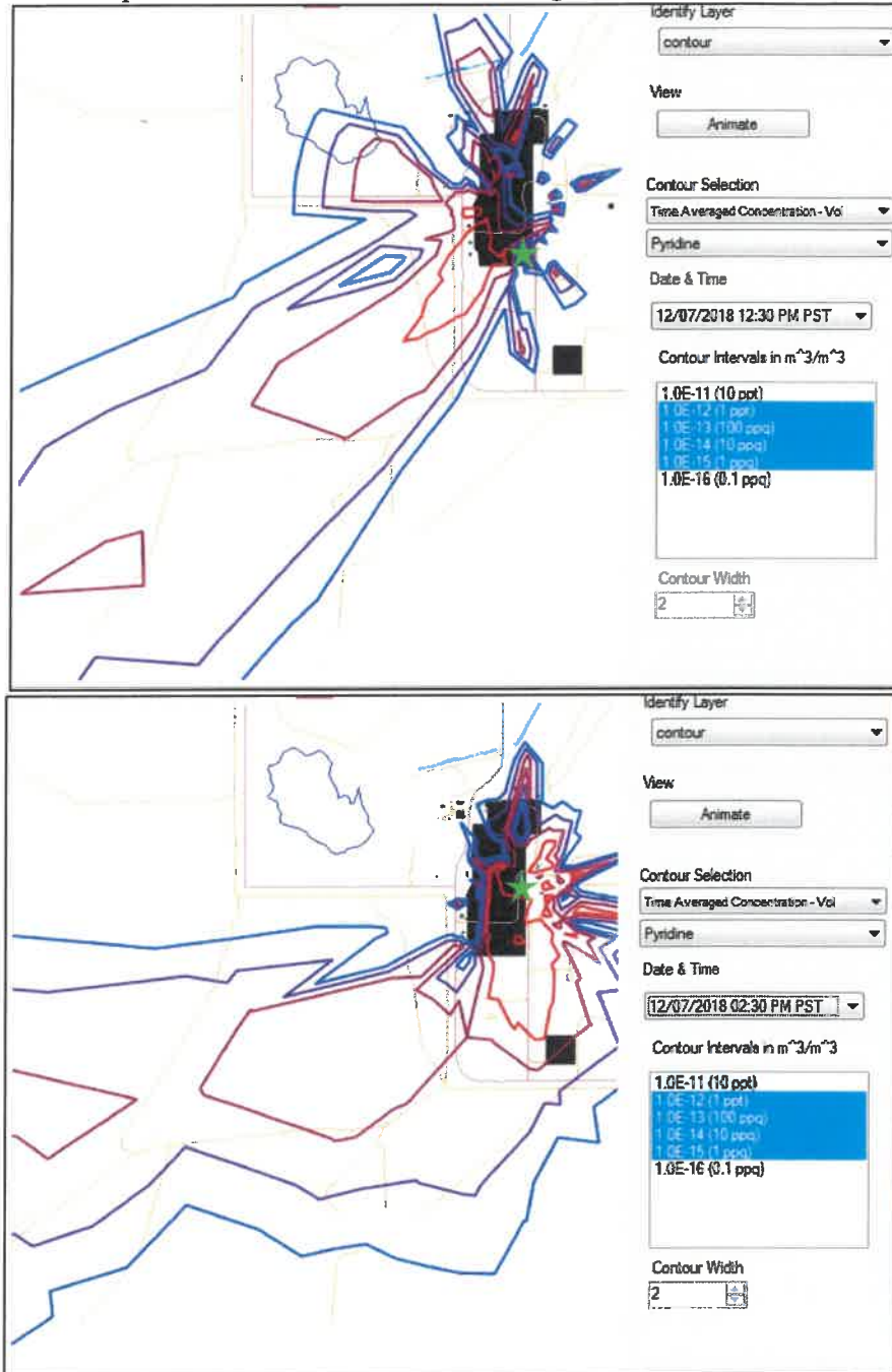
Figure 2. APGEMS-TF plume estimates from 12:30 (upper panel) and 2:30 (lower panel) assuming conservatively high releases of pyridine from each of the SX, S and SY-Farm PBFs. AOP-15 locations identified with light green stars.
