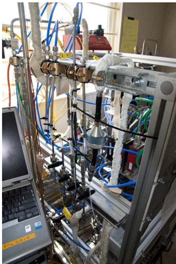
Figure B.19. The north side of the gas control rack included the sorption tube sample collection system. Some of the things not shown were the heat tape controllers for the FTIR, PTRMS, heated soot filter, nitrogen preheater, water vaporizer, and exhaust lines from the VAU.
