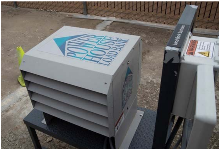
Figure A.11. The Powerhouse Manufacturing (model 11.3-.25-240-1) switch box and 11.25 kVA load bank. This is switched to the full 11.25 kVA load during steady state testing on the diesel engine.
