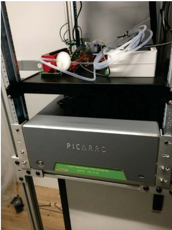
Figure 5. Picarro Ammonia Analyzer for the New Mobile Laboratory (Photo courtesy of G. Weeks.)
