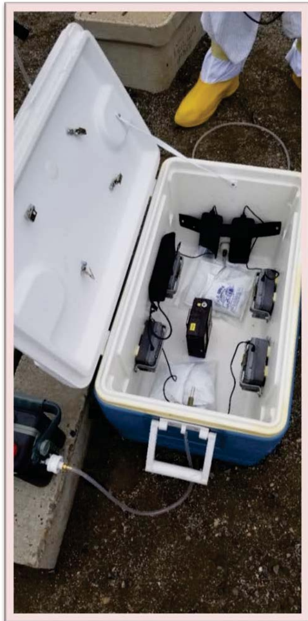
Figure 7. (Right) Four C2Sensors with Sample Pump and Ice Packs to Maintain Temperature. (Photo courtesy of E. Morrey.)
