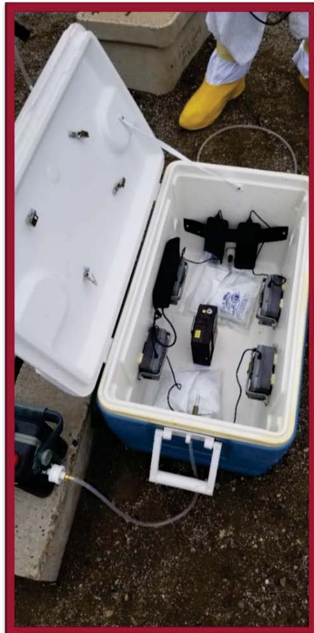
Figure 6. (Left) Sample Pump Tubing Running to A-103 HEPA Filter. (Photo courtesy of E. Morrey.)
