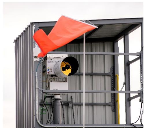
Part of an optical spectrum gas imager installed at AP Farm.
