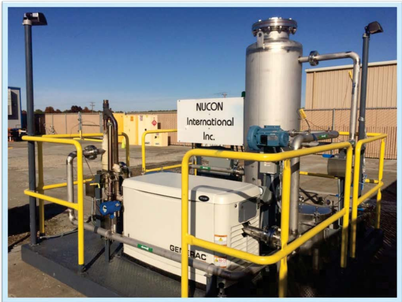
Located at Pacific Northwest National Laboratory is the NUCON Vapor Abatement Unit (VAU) prototype where it will undergo bench-scale testing. For more details, read KPP 4 . (Photo courtesy of E. Morrey)
