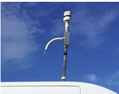
Figure 2-3. The sampling mast used for the mobile real time plume chasing.
