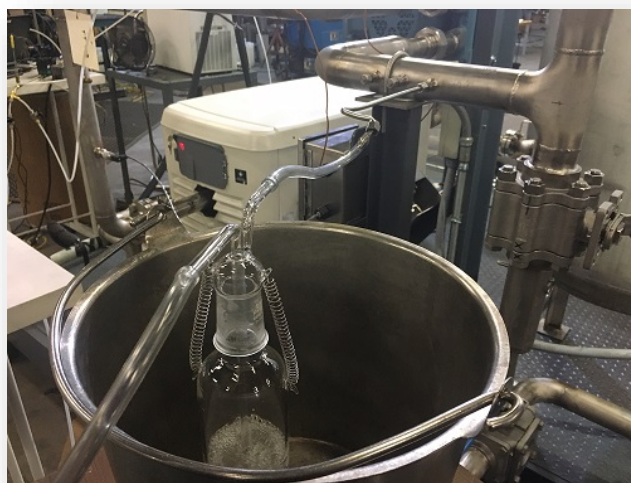
NUCON Lab System that Generates Vapors
